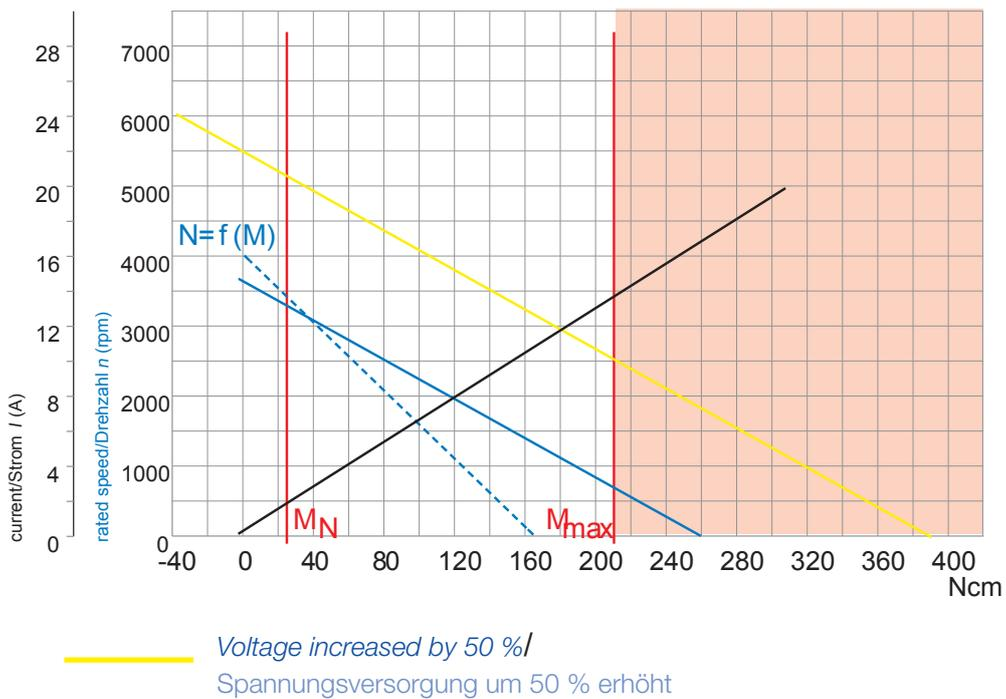
In combination with corresponding speed controllers, the speed drop can be compensated, and the speed remains constant even with increasing load.
